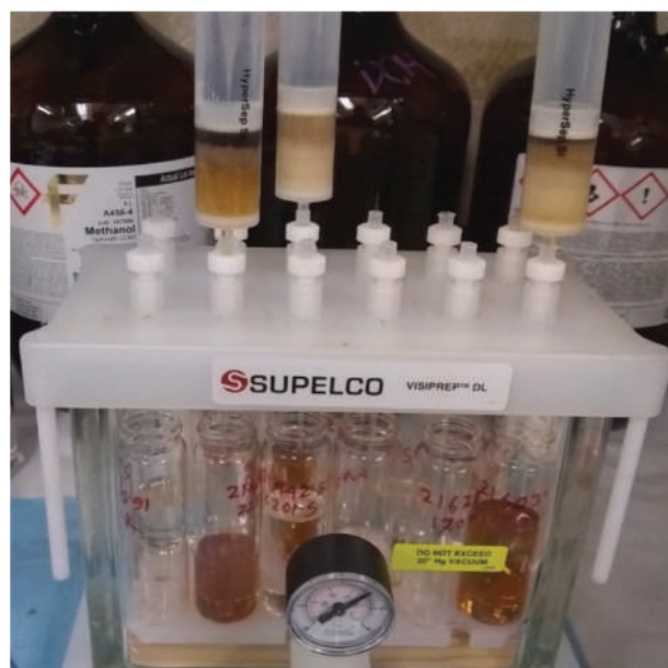
Fig. 2. The small scale apparatus developed for SARA fractionation (reprinted from [49]).
