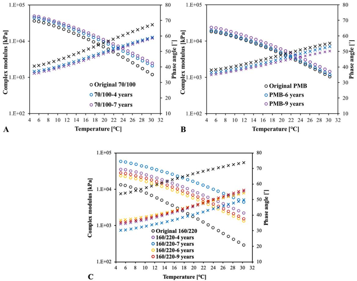
Fig. 4. The complex modulus and phase angle of bitumen (A: 70/100 of surface layer; B: PMB of surface layer; C: 160/220 of base layer).
