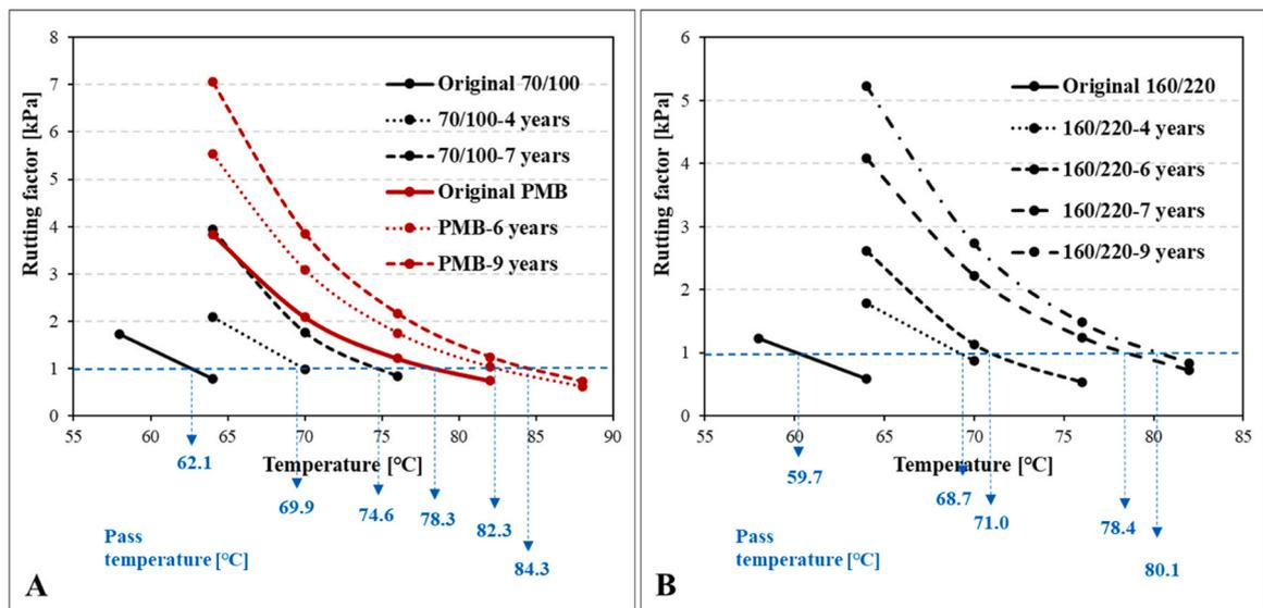
Fig. 5. The performance grade evaluation of bitumen (A: surface layer bitumen (70/100 and PMB); B: base layer bitumen).
