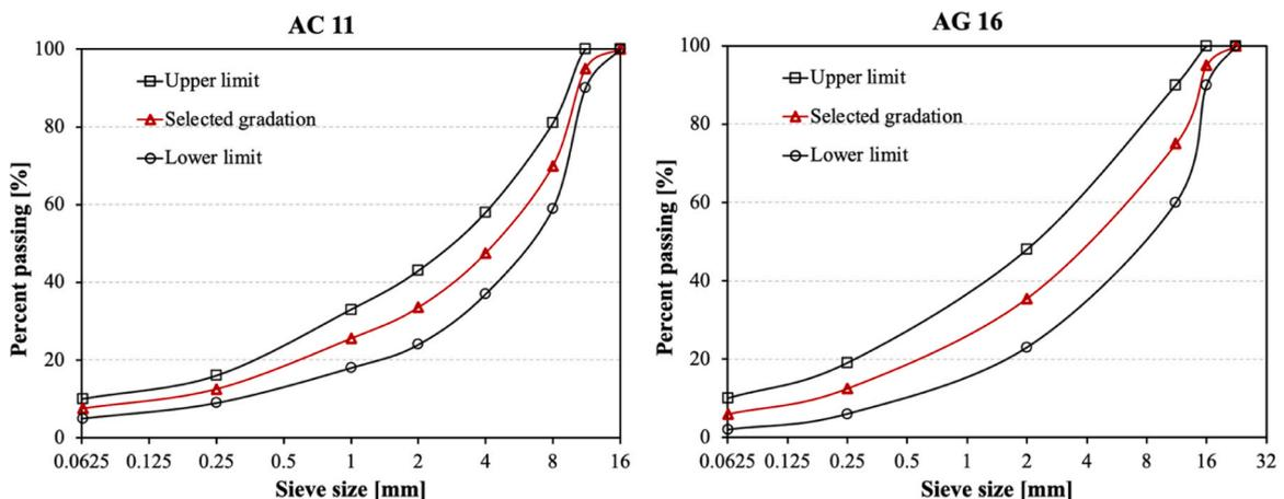
Fig. 1. Aggregate gradation for AC 11 (left) and AG 16 (right).
