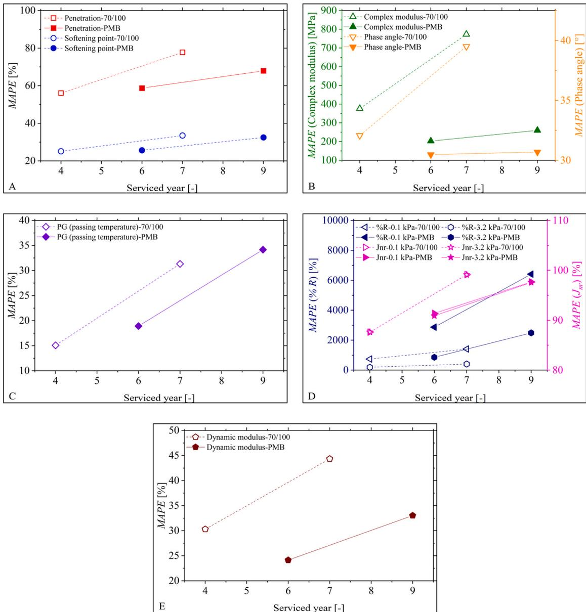
**Fig. 8.** MAPEs of difference performance after ageing for base layer bitumen 160/220: (A) physical properties, (B) rheological properties, (C) PG, (D) creep recovery properties and E dynamic modulus.
