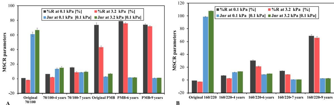
Fig. 6. %R and  $J_{nr}$  of surface (A) and base (B) layer bitumen.
