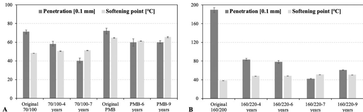
Fig. 2. Physical parameters of surface layer bitumen (A) and base layer bitumen (B).
