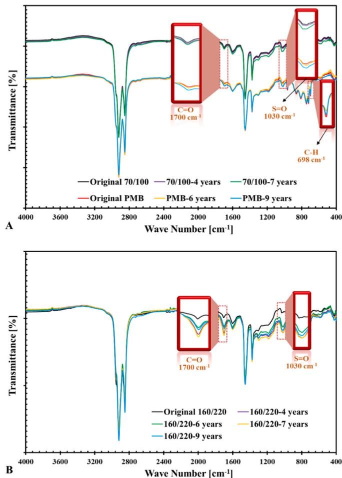
Fig. 3. The FTIR spectra of bitumen (A: PMB and 70/100 of surface layer; B: 160/220 of base layer).
