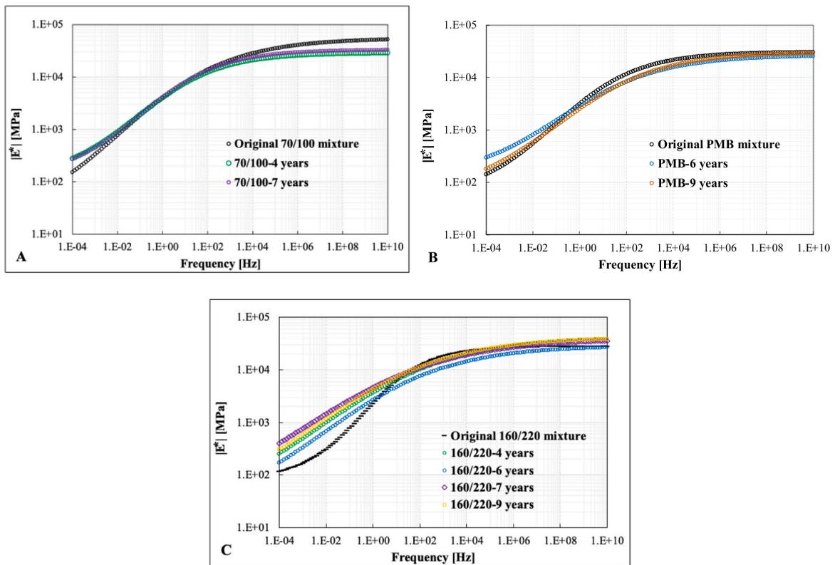
Fig. 7. The master curve of surface (A and B) and base layer mixtures (C).
